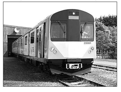
The Class 230 *(Left)* has been designed as a cost-effective solution to over-crowding on the rail network. The train costs considerably less to acquire and run, about a third less than a comparable unit, and uses about a third less fuel. The ground-breaking engine modules allow the train to be maintained trackside, rather than needing to return to a depot.
